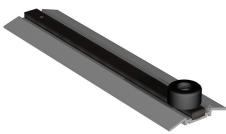
**FLAT TRACK END STOPS**: Standard track end stop is 1-1/2" diameter rubber cushion reinforced with an internal steel washer. End stop attached at each end of track run through pre-drilled factory hole with Hilti II  $\frac{1}{4}$ " x 3-1/4" anchor. The end stops prevent the carriages from running off of the track.
