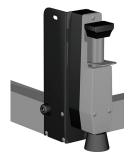
**ANTI-DRIFT MECHANISM**: The anti-drift mechanism secures carriage in place and prevents the carriage from drifting. The securing mechanism is engaged by simply pressing down the shaft with your foot and is released by flipping the tab up with your foot.
