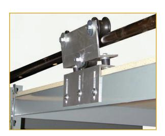
Overhead Anti-Tip (OHAT) includes a flexible mounting bracket and a roller guide to secure mobile systems overhead. The OHAT eliminates additional floor track by attaching to the top of the shelving instead of to the carriage base. Additionally, Overhead Anti-Tip flexes vertically to allow freedom of movement on irregular floors. The triple roller bracket provides an ease of movement while securing the carriages against tipping.
