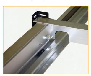
"Z" Rail Anti-Tip includes two anti-tip brackets which are mounted on the carriage wheel channel. As the carriage moves back and forth, these brackets slide in the open portion of the floor mounted "Z" Rail. The "Z" Rail stands upright 1" and is not ADA compliant. The "Z" Rail anti-tip option is compatible with all Pipp carriage families.
