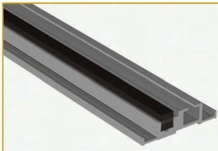
**Decked ITAT Flat Track** overall is 4-5/8" wide and 1-5/16" high. When installed, only 1/8" of the 7/8" X 3/4" steel insert is above the decking. This track is primarily used when specifications require a levelable track. This track was designed with high grade engineered composite decking in mind. This will provide a completely "finished" look to the overall system. The track is ideal for heavy duty carriages like mechanical-assist and electric carriages.
