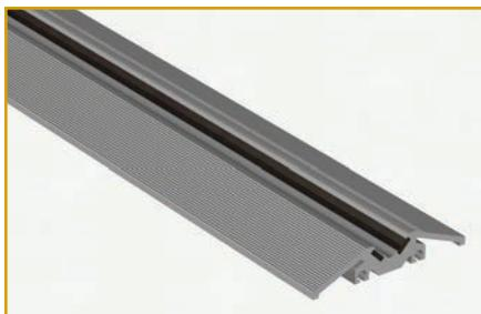
**Non-Adjustable Heavy Duty Manual "V" Groove Track** is less than 2-3/4" wide, 1/2" at its highest point and is made from heat treated aluminum. There is no adjustability within the track for this style but this track can be leveled through shimming. This track can be used with the standard manual carriage, provides a price competitive heavy duty track option. The Non-Adjustable Heavy Duty Manual "V" Groove Track is compatible with all In-Track Anti-Tip Tracks.
