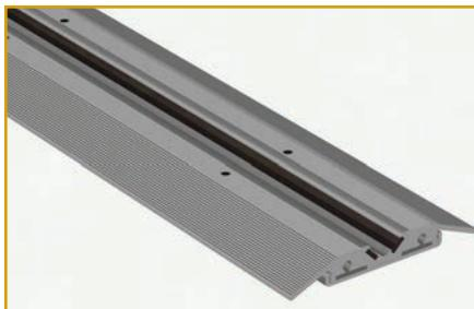
**Adjustable Standard Manual "V" Groove Track** is just over 3-1/4" wide, less than 7/16" at its highest point and is made from heat treated aluminum. This adjustable track has set screws which allow for a 1/4" of leveling if needed and is available with flat or carpet "grabbing" underlayment. This track can be used with the standard manual carriage.
