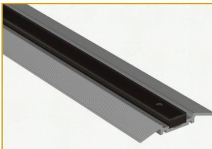
**Heavy Duty Flat Track** is less than 3-1/4" wide, 1/2" at its highest point and is made from aluminum. It has a flat steel insert that is 3/4" wide. This track will eliminate debris in the groove. There is no adjustability within the track for this style but this track can be leveled through shimming. This track can be used with the heavy duty flat track carriage and the mechanical-assist carriage.
