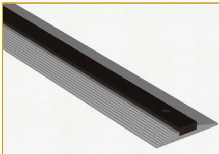
**Standard Flat Track** is 2-1/4" wide, 3/8" at its highest point and is made from heat treated aluminum. It has a flat steel insert that is 5/8" wide in place of the "V" groove. This will reduce debris in the track. There is no adjustability within the track for this style but this track can be leveled through shimming. This track can be used with the standard flat track carriage.
